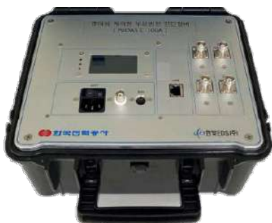
Partial discharge diagnosis device for high-voltage cables in a live status
